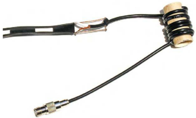
Figure 2 — The J-pole feeding end is on the lower left, and the choke is on the right. [Fred Delaney, K1DU, photo]
