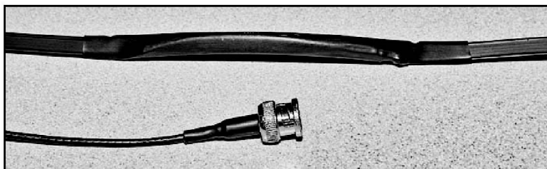
Figure 5 — The \lambda/4 UHF decoupling stub made of RG-174A, covered with heat shrink tubing. This is shown next to the BNC connector that goes to the transceiver.
